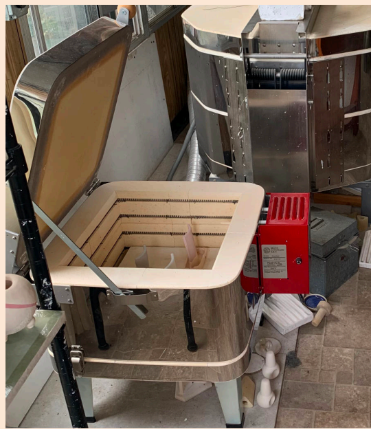
Skutt GlazeTech test kiln, $1767. Genesis mini Touch Screen Nearly new, lightly used. Perfect for glaze testing 12" deep, 14.5"x14.5" 2 shelves, 13"x14" various bead racks and test tile holders
